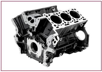
The VM Motori 3.0 litre V6 cylinder block and bedplate, used in Chrysler, Jeep and Lancia vehicles, in series production at the Tupy foundry in Brazil since 2010 (Courtesy VM Motori)
