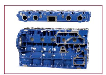
The Ford Ecotorq 7.0 and 9.3 litre commercial vehicle cylinder block and head, in series production at the Componenta foundry in Turkey since 2007 (Courtesy Ford-Otosan)
