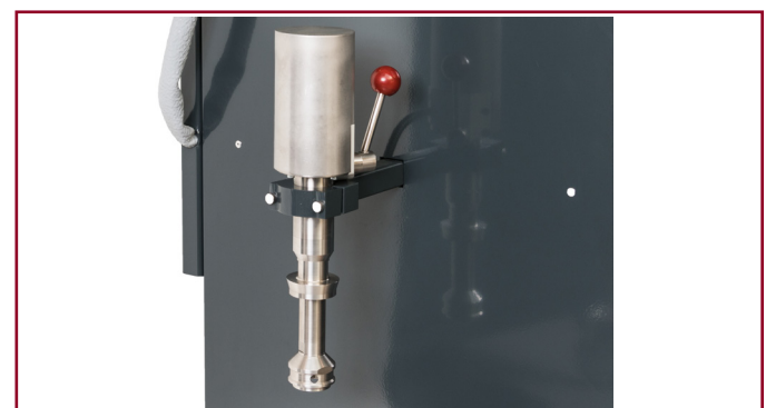
Figure 3: Re-engineered SAM with improved Thermocouple Holder
