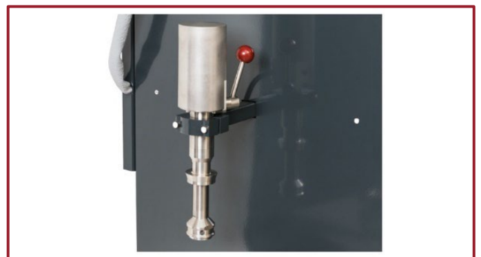
Figure 3: Re-engineered SAM with improved Thermocouple Pair Holder
