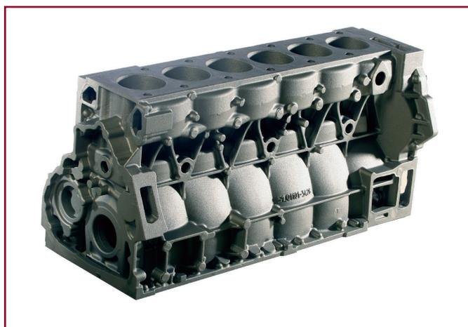
*The Navistar MaxxForce™ 11 and 13 cylinder block, in series production at the PurePOWER foundry in the USA since 2011 and at the Tupy foundry in Brazil since 2008 (Courtesy Navistar)*
