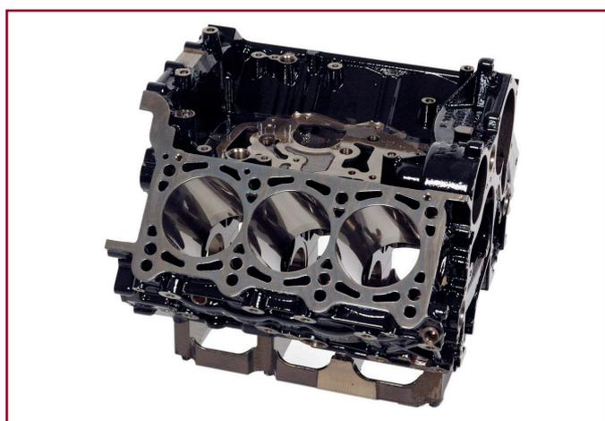
*The Audi 3.0 litre V6 cylinder block, used in Audi, Porsche and Volkswagen vehicles, in production at the Tupy foundry in Brazil since 2003 (Courtesy Audi)*
