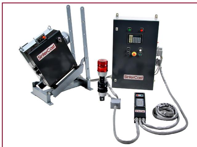
The Complete Wirefeeder, including Wirefeeder Head, Control Cabinet, Operator Box and Signal Lamp Assembly
