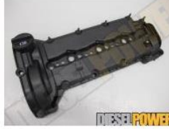
Plastic valve covers are used to reduce weight and provide a layer of sound insulation in the engine.
