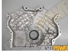
The engine's three-piece front cover is cast aluminum, and it ties the front of the engine to the chassis.
