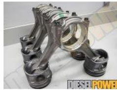
These connecting rods feature Cummins-like rod caps that are so large their parting lines
