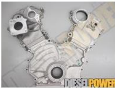
As installed on the engine, the cover acts as a mounting system for the injection pump, valve train, and other components.
