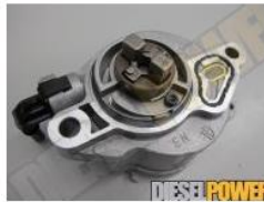
For vehicles that need vacuum to run the climate controls or brake system, the 3.0L can be equipped with a vacuum pump.
