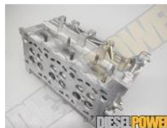
From this angle, you can see the siamesed exhaust ports, and the area where the injectors
