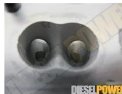
Even as cast from the factory, the ports have very smooth and consistent shapes that are f
