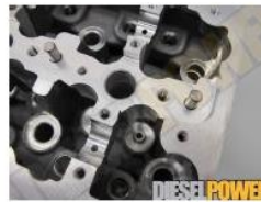
The engine uses Bosch CRIN 3.4 injectors that are clamped through the valve covers using t
