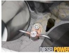
Each of the cylinders is equipped with its own oil jet to cool the bottom of the pistons.
