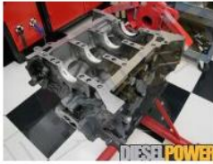
When flipped over, you can see the large main-bearing webs that are cast into the reinforce
