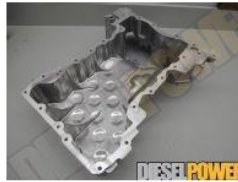
The 3.0L's oil pan is a piece of cast-aluminum beauty. Using aluminum aids in cooling the
