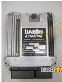
Getting an all-new engine like this to run in a standalone configuration requires a special electronic control system.
