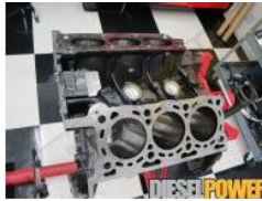
The 630T's 60-degree V-6 block is made from high-strength compacted-graphite. On an engine
