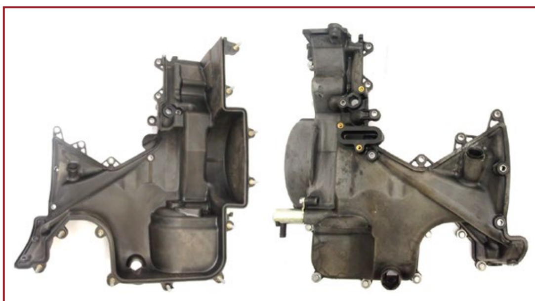
Figure 8: Inner and outer surfaces of the left-side plastic casings at the conclusion of the 100-hour engine test
