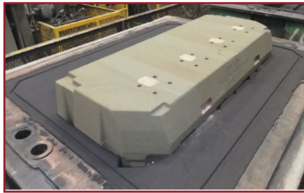
b) Assembled core package with four ladderframes set into standard series production green sand flask
